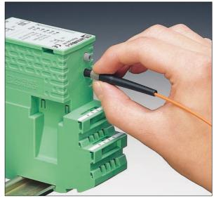
Push the polymer fiber through the plug connector.
