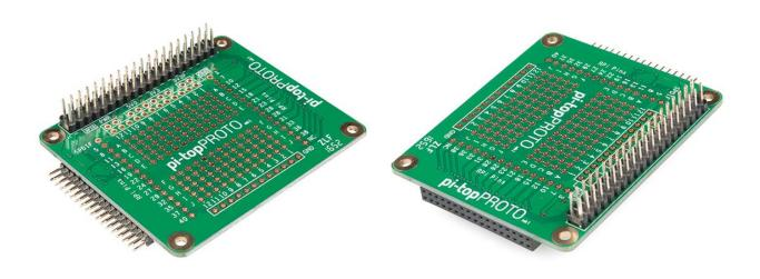
**Description:** The pi-topPROTO is a HAT-compatible add-on board for prototyping electronics for your pi-top or pi-topCEED. With plenty of space available to build circuits that can interact with your pi-top — as well as a full 40-pin GPIO on top for a desired Raspberry Pi HAT — the pi-topPROTO makes a great addition to the pi-top family.
