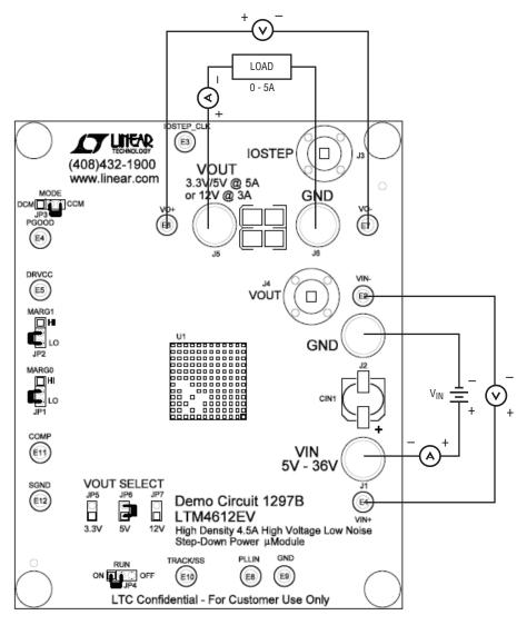
Figure 1. Test Setup of DC1297B
