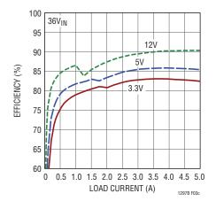
Figure 3. Measured DC1297B Efficiency at 12V<sub>IN</sub>, 24V<sub>IN</sub>, 36V<sub>IN</sub> (DCM mode enabled)
