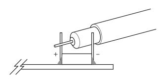
Figure 2. Scope Probe Placements for Measuring Input or Output Ripple
