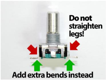
You need to be **REALLY** CAREFUL when doing this. DO **NOT** straighten the existing bends — the legs will crack off! Instead, add extra bends a little further down.
