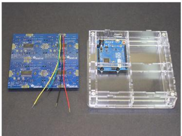
SDA from Trellis to SDA on Arduino (this is the second pin, next to SCL)
