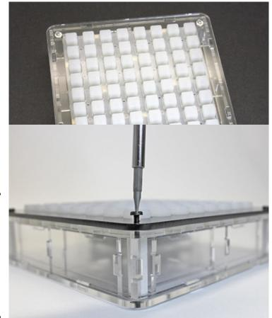
Install four corner screws through both top waffles and into the standoffs.
