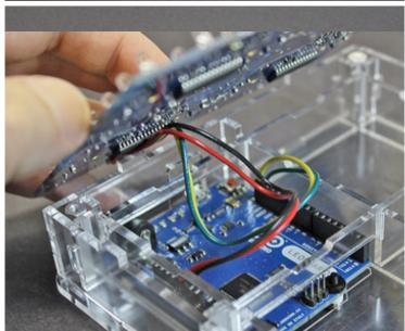
Now the Trellis gets turned over, LED side up, and is lowered into place in the case. You'll see the horizontal and vertical braces have notches into which the board neatly fits.
