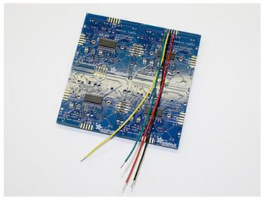
Trellis boards...with the text upright, in the normal orientation for reading...connect the wires to the header along the **top edge**, toward the **right**. They should be about 6 inches (15 cm) long, or a little longer.
