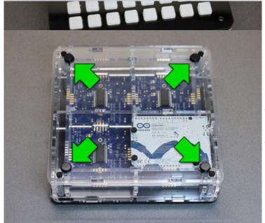
Turn the whole thing over and peel-and-stick the four rubber feet near the corners.
