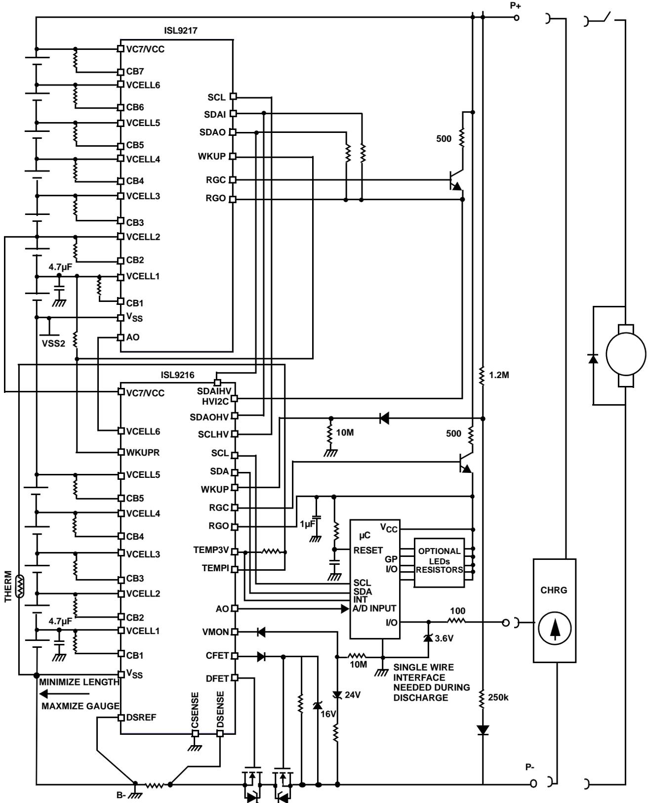
FIGURE 17. 12-CELL CASCADED APPLICATION CIRCUIT WITH INTEGRATED CHARGE/DISCHARGE
