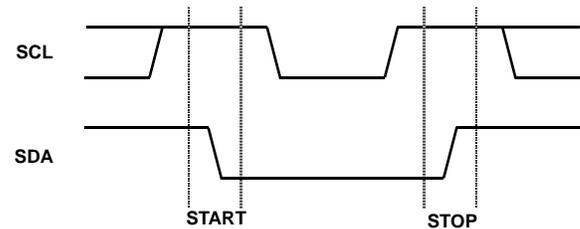
FIGURE 10. I<sup>2</sup>C START AND STOP BITS
