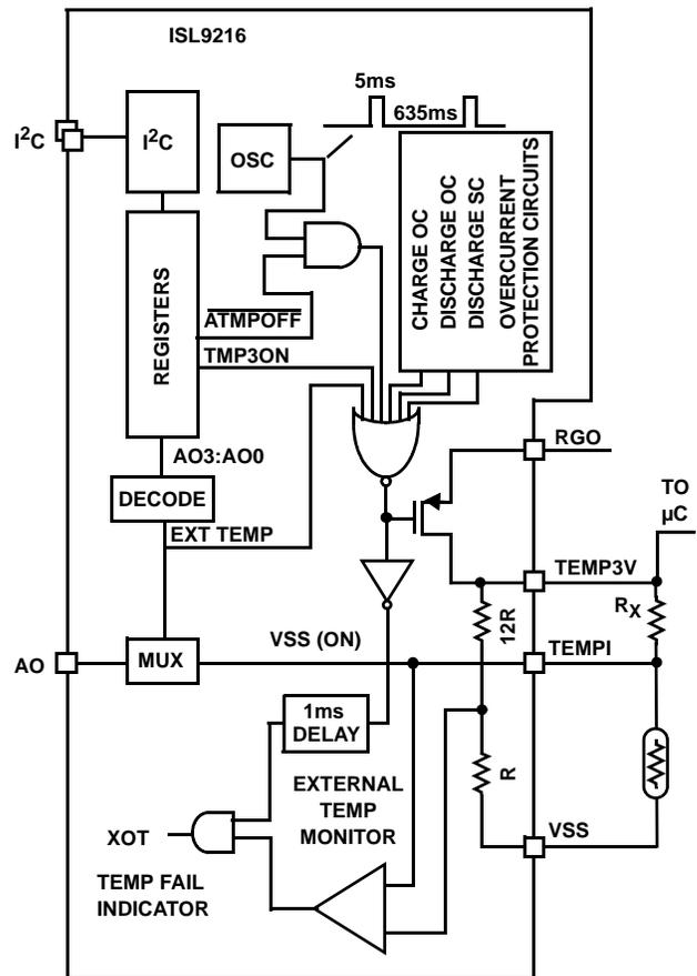
FIGURE 5. EXTERNAL TEMPERATURE MONITORING AND CONTROL (ISL9216 ONLY)
