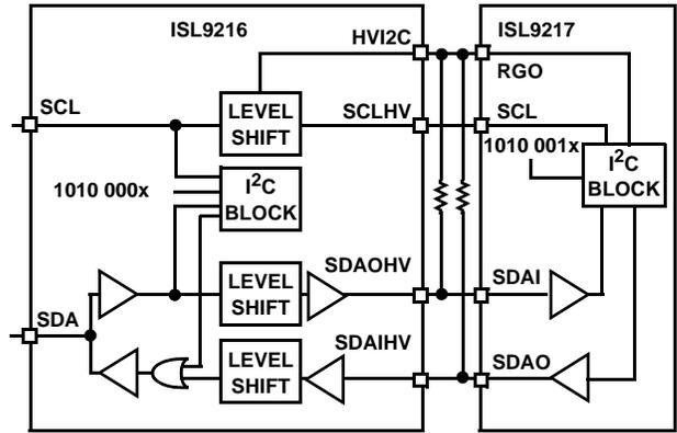
FIGURE 15. I<sup>2</sup>C CASCADED INTERFACE
