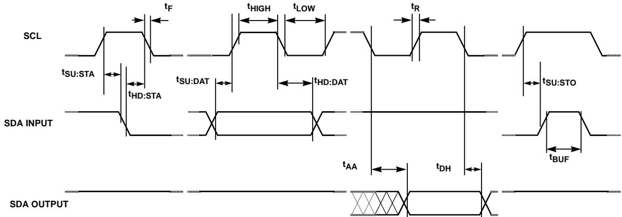
This timing shows the communication with the ISL9216. Communication with the ISL9217 (through the ISL9216) adds some lag time, however, overall the communication with the ISL9217 meets the same timing requirements as communication with the ISL9216.
