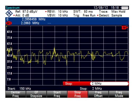
Figure 22. Conducted EMI Pre-compliance 150 kHz-2 MHz
