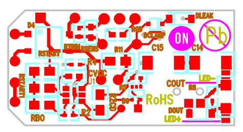
Figure 8. Solder Side PCB
