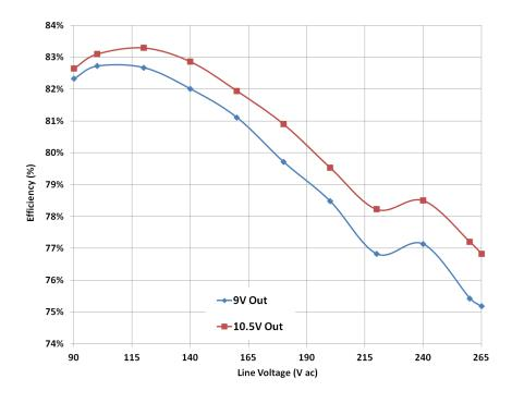
Figure 15. Efficiency over Line Voltage
