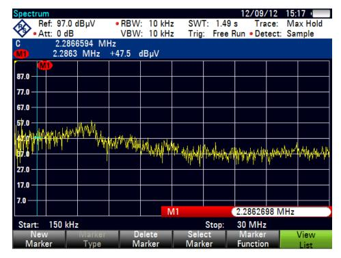
Figure 23. Conducted EMI Pre-compliance 150 kHz-30 MHz
