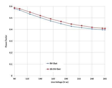
Figure 16. Power Factor over Line Voltage
