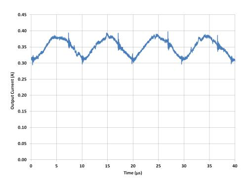
Figure 20. Output Ripple 90 V ac 50 Hz
