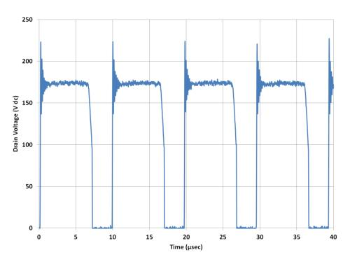
Figure 18. Drain Voltage @ 90 V ac
