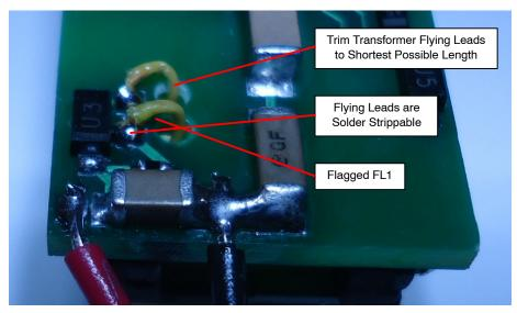
Figure 12. Transformer and Output Terminations
