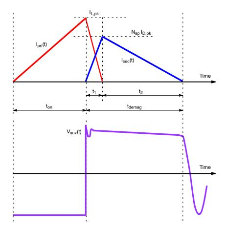
Figure 3. Flyback Currents and Auxiliary Winding Voltage in DCM
