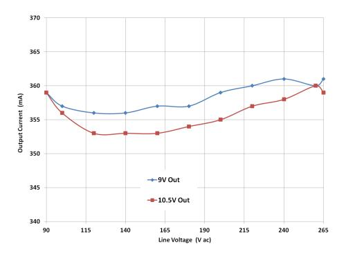
Figure 14. Regulation over Line Voltage
