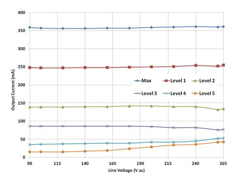
Figure 17. Dimming over Line Voltage
