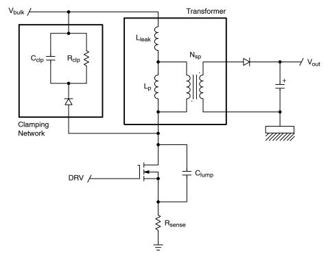
Figure 2. Basic Fly-back Converter Schematic
