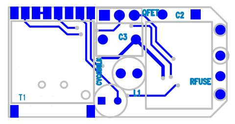
Figure 6. Component Side PCB
