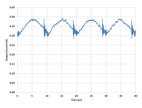
Figure 21. Output Ripple 265 V ac 50 Hz
