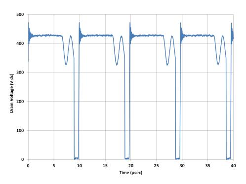
Figure 19. Drain Voltage @ 265 V ac
