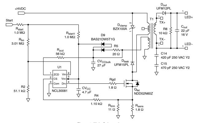
Figure 5. Main Schematic
