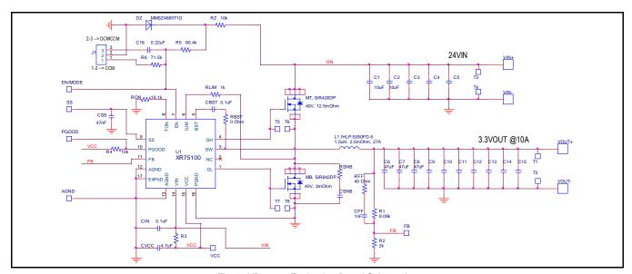
Fig. 1: XR75100 Evaluation Board Schematics
