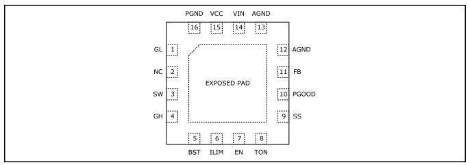
Fig. 2: XR75100 Pin Assignment
