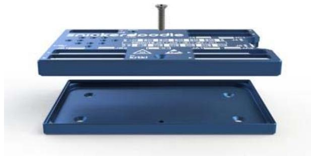
Don't let your cookies get stale... keeps your snickerdoodle safe, clean, cool, and securely mounted in your autonomous cat-herding robot. cookieJar's are machined out of 6061 aluminum, bead blasted, anodized, and laser engraved. They've got an internal boss + thermal pad so the enclosure will act as the heat sink! There are four countersunk mounting holes in the base if you want to strap this thing to whatever you're driving/flying around... We'll provide the screws.
