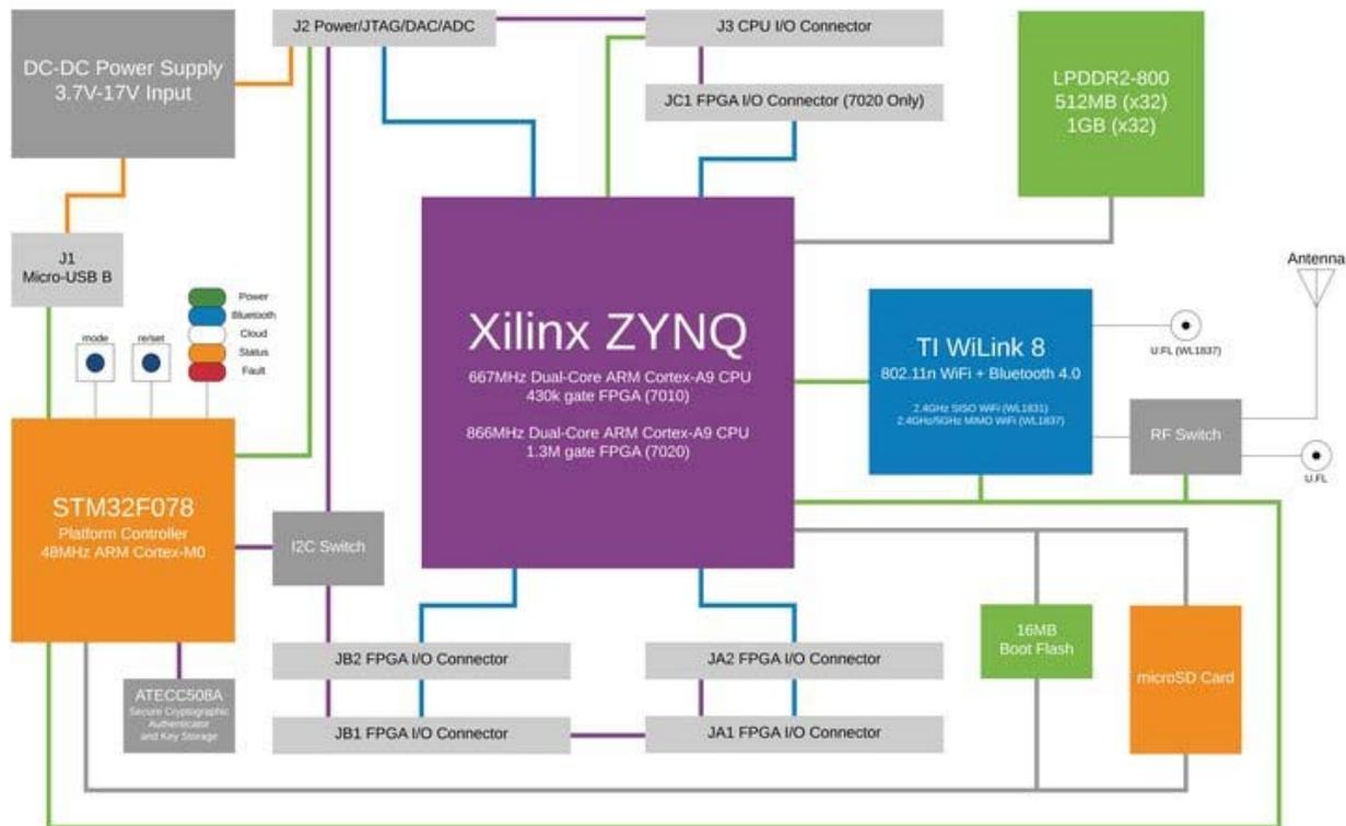
Below are the high-level technical specifications for snickerdoodle (items in **bold** are configuration specific):
