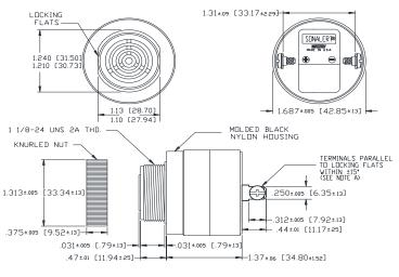
NOTE A: TERMINALS-.032 BRASS TIN PLATED, TAPPED FOR #6-32 SCREW. TWD #6-32 NICKEL PLATED BRASS SCREWS INCLUDED. WILL ACCEPT 1/4\* QUICK CONNECT.
