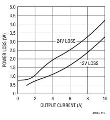
Figure 15. 3.3V Power Loss Curves vs Load Current
