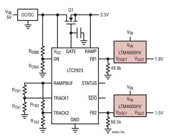
Figure 6. Output Voltage Tracking with the LTC2923 Controller
