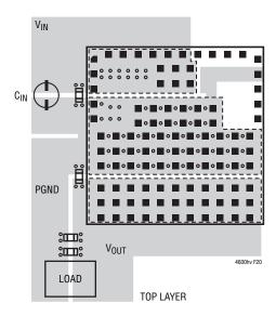
Figure 20. Recommended PCB Layout
