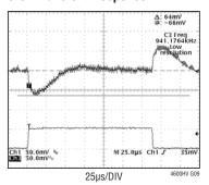
3.3V AT  $5A/\mu s$  LOAD STEP  $C_{OUT} = 3 \bullet 22\mu F$  6.3V CERAMICS  $470\mu F$  4V SANYO POSCAP C3 = 100pF
