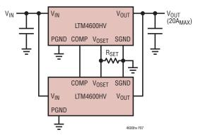
Figure 7. Parallel Two µModules with Load Sharing
