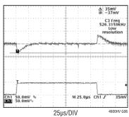
1.5V AT 5A/µs LOAD STEP C<sub>OUT</sub> = 3 • 22µF 6.3V CERAMICS 470µF 4V SANYO POSCAP C3 = 100pF
