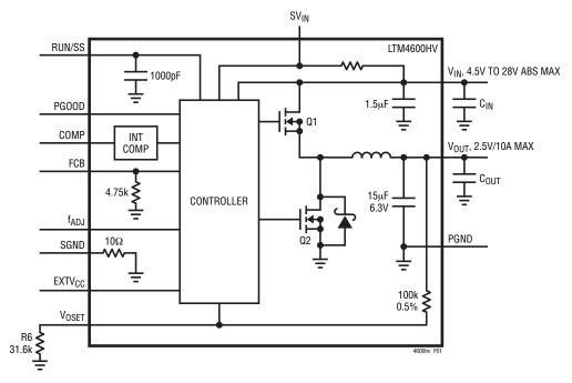
Figure 1. Simplified LTM4600HV Block Diagram
