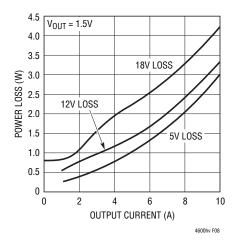
Figure 8. 1.5V Power Loss Curves vs Load Current
