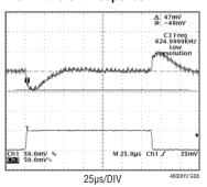
2.5V AT 5A/µs LOAD STEP C<sub>OUT</sub> = 3 • 22µF 6.3V CERAMICS 470µF 4V SANYO POSCAP C3 = 100pF
