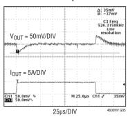
1.2V AT 5A/µs LOAD STEP C<sub>OUT</sub> = 3 • 22µF 6.3V CERAMICS 470µF 4V SANYO POSCAP C3 = 100pF
