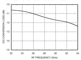
Note 1: Single side band measurement without 90° hybrid, and second IF port terminated.
