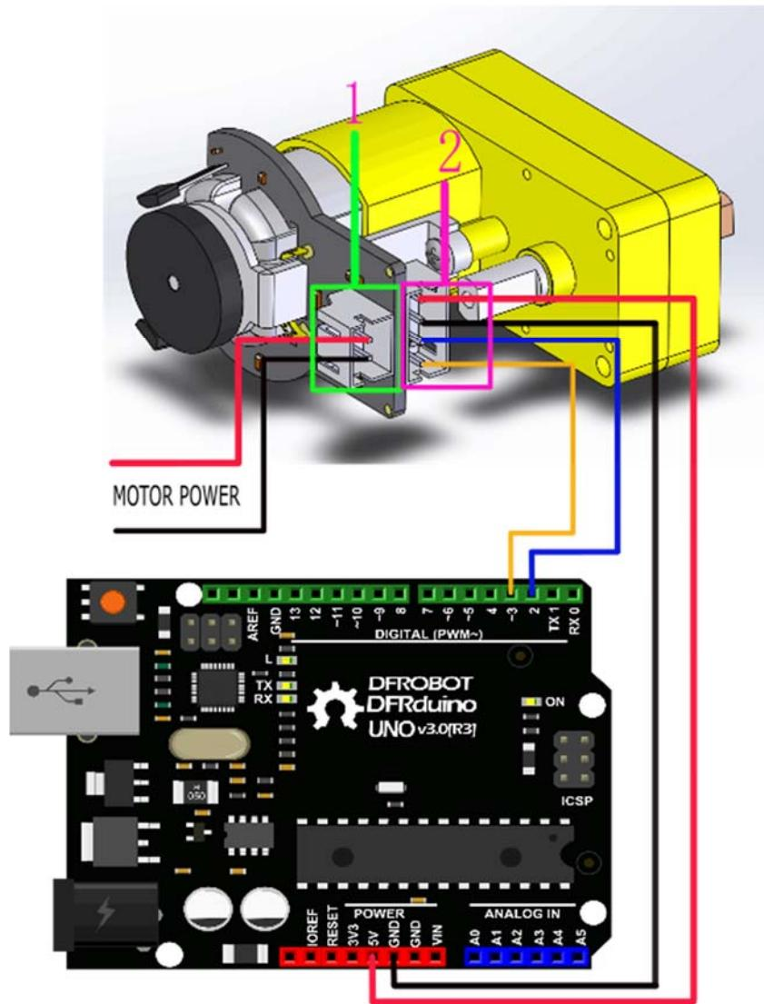
This tutorial is intended to use the encoder. Select D2 pin and D3 pin, Wherein D2 as an interrupt port, D3 as an input pin. In practice, two pins need to ensure that one of pins must be an interrupt pin, and the other definable (see the interrupt port with different board).
