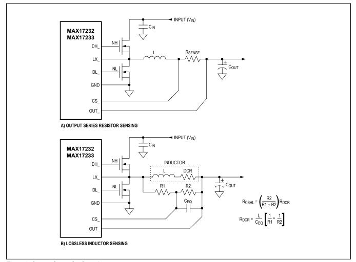
Figure 1. Current-Sense Configurations
