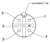
To put device in programming mode: Connect Mode pin #1 to GND @ Power up. Leave Mode pin #1 open for run mode (Normal Operation)
