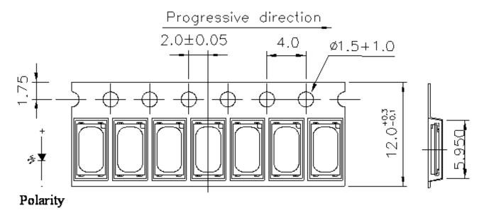
Note: Tolerances unless mentioned ±0.1mm. Unit = mm
