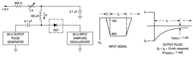
1. A 2.0 k $\Omega$  variable resistor adjusted for a Forward Current (IF) of 10 mA.
