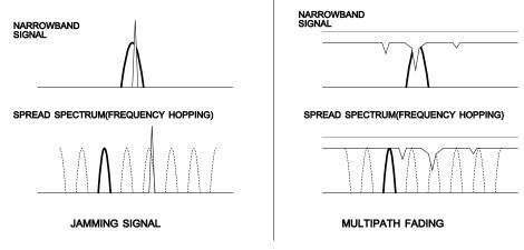
Narrow-band versus spread-spectrum transmission Figure 1.1.1
