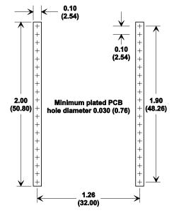
Connectors are FCI Electronics 75915-420LF or equivalent Dimensions in inches and (mm)
