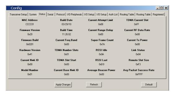
Figure 5.6.2.4 shows the *Status* tab contents, corresponding to Bank 2. Note the *Status* tab contains read-only parameters.
