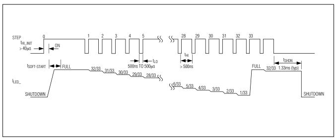
Figure 1. MAX8901B Timing Diagram
