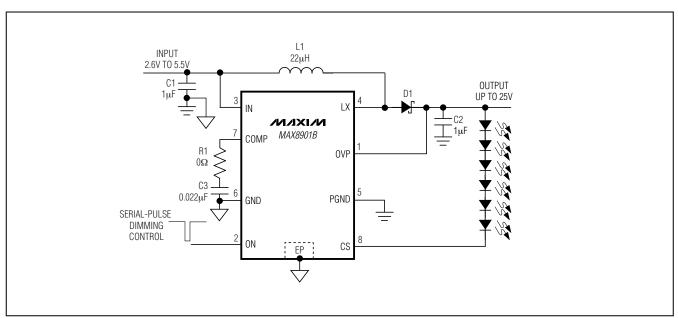
Figure 5. MAX8901B Application Circuit
