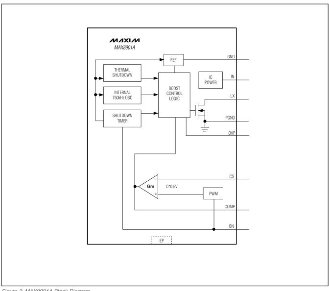
Figure 2. MAX8901A Block Diagram
