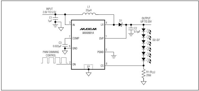
Figure 4. MAX8901A Application Circuit
