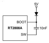
Figure 2. External Bootstrap Diode
