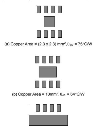
(c) Copper Area =  $30 \text{mm}^2$ ,  $\theta_{JA} = 54^{\circ}\text{C/W}$
