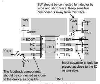
Figure 5. PCB Layout Guide
