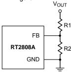
Figure 1. Output Voltage Setting
