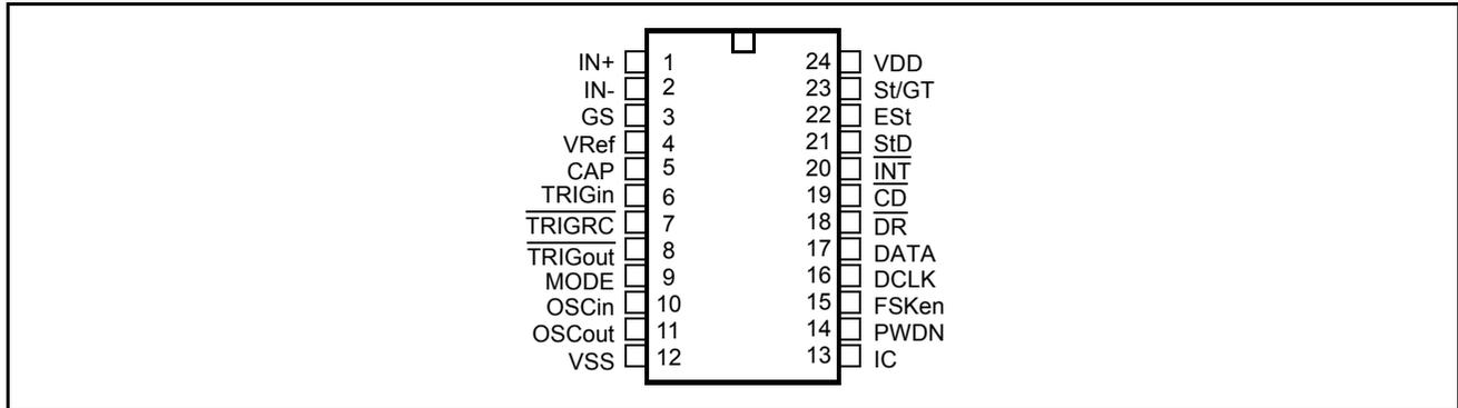
Figure 2 - Pin Connections
