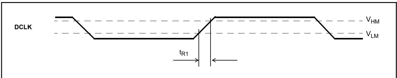
Figure 15 - DCLK Mode 1 Input Timing
