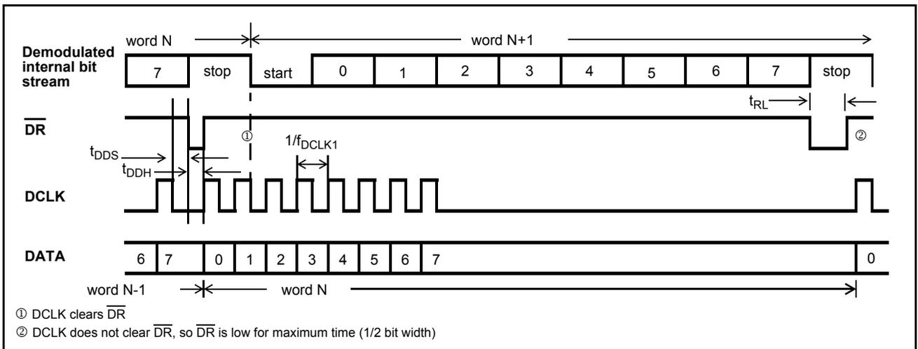
Figure 16 - Serial Data Interface Timing (Mode 1)
