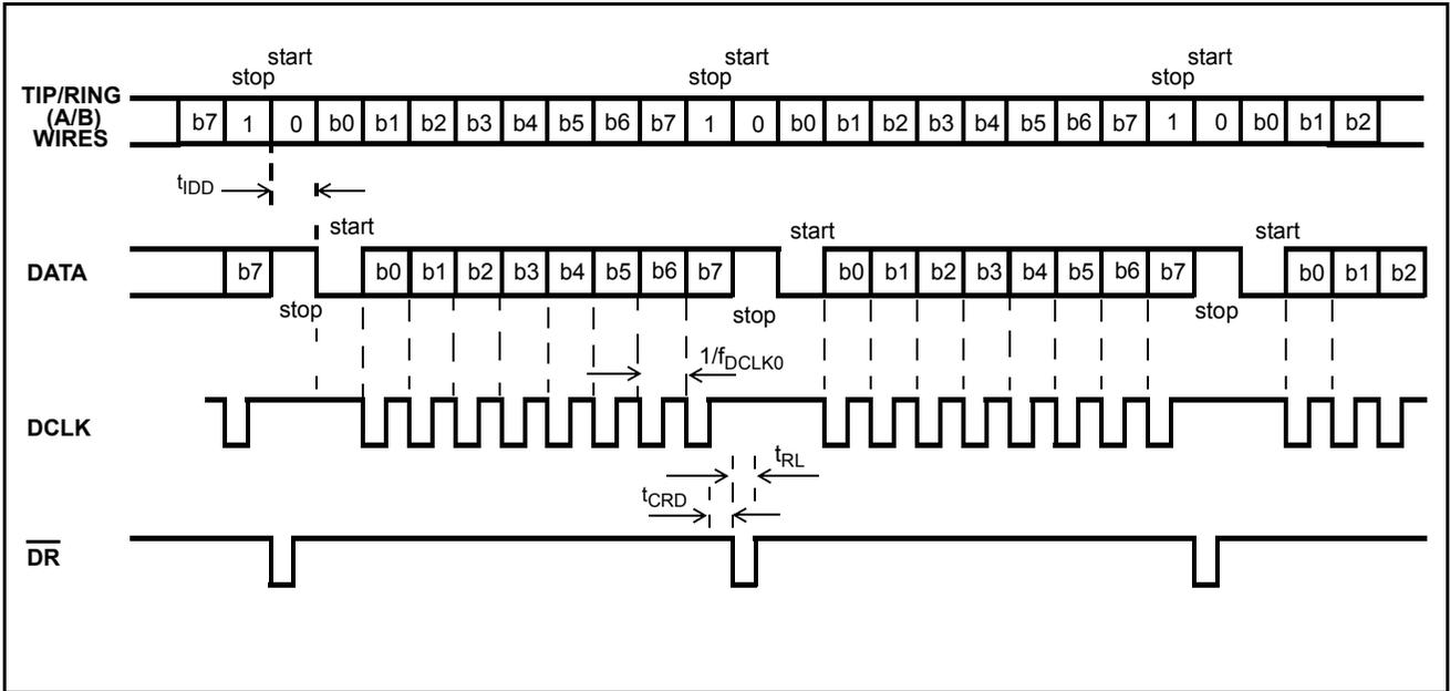
Figure 14 - Serial Data Interface Timing (MODE 0)
