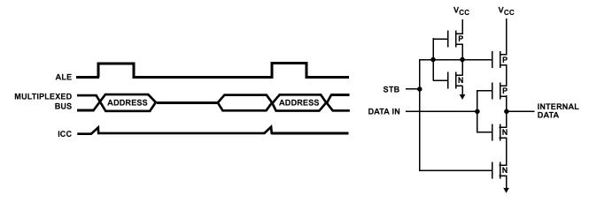
FIGURE 18. SYSTEM EFFECTS OF GATED INPUTS
